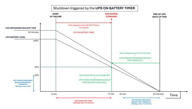
The timer can be set in seconds or minutes using unit 's' or 'm' in the parameter value:
