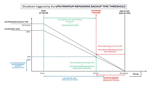
This threshold is being set in minutes (m) in the parameter value:
