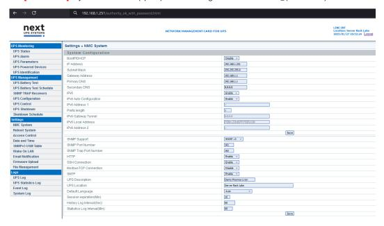
After configuring the UPS IP address, up to 2 UPSs can be monitored in the PPM, if two UPSs are configured both will be monitored simultaneously for executing the shutdown settings. See chapter 4.2.3 SHUTDOWN CONFIGURATION for more information on the shutdown configuration.
